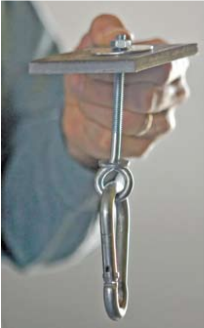
Flat Load Test Block
